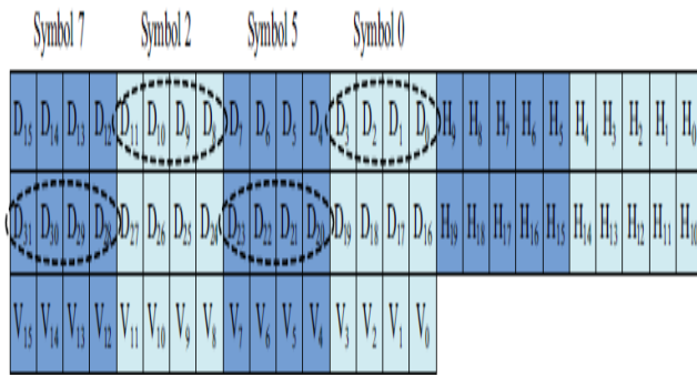
Fig: 2 32 bit word can be divided as 8 symbols with k=2 \times 4 and m=4 .
