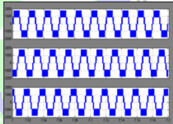
Fig.9Five-level-inverter output voltages of three phases.
