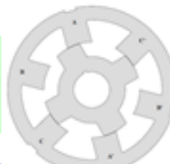
Fig.6 – Phase A missing 15 graus to aligned in a TPSRM.
