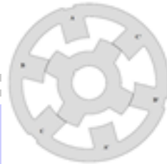
Fig.5 –Phase A completely disaligned in a TPSRM.
