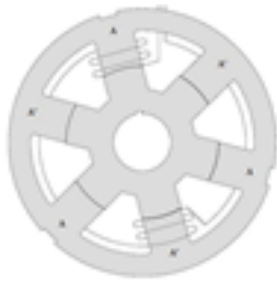
Fig.2 –Cross Section of a SPSRM, showing a part winding of the phase A.
