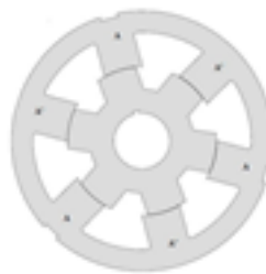
Fig.10 – Phase A missing 5^\circ to aligned in a SPSRM.
