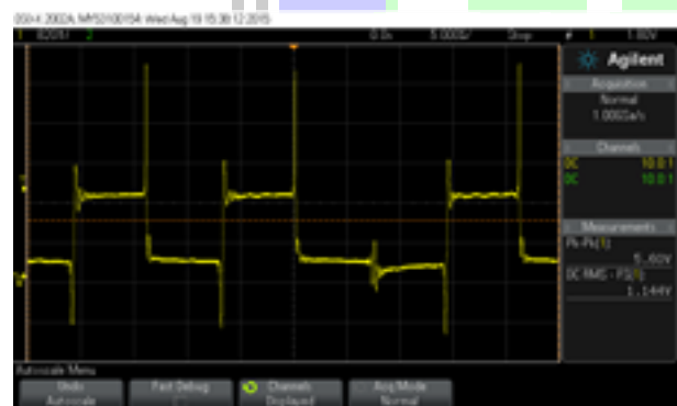
Figure 17: Voltage stress across S_a
